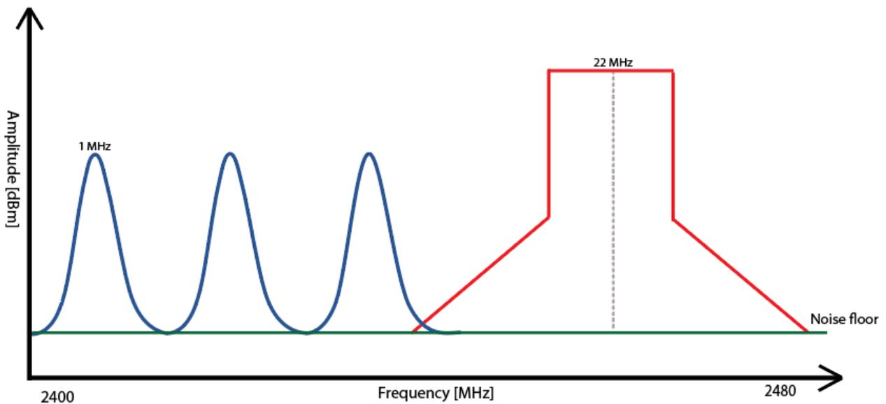
Figure 6: Narrowband signals co-existing with WiFi
