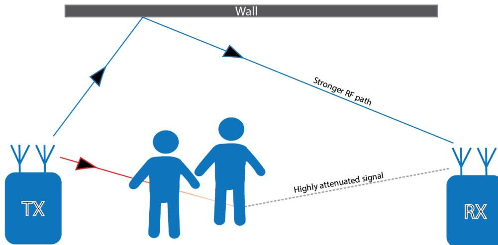
Figure 4: Direct RF path blocked by bodies
