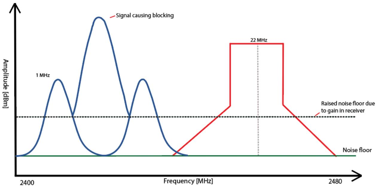
Figure 7: Receiver blocking scenario
