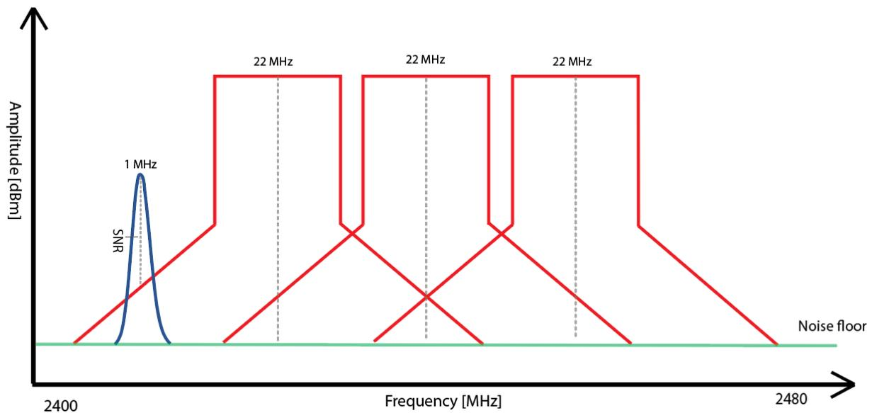
Figure 5: Narrowband signal with reduced SNR due to WiFi sidebands
