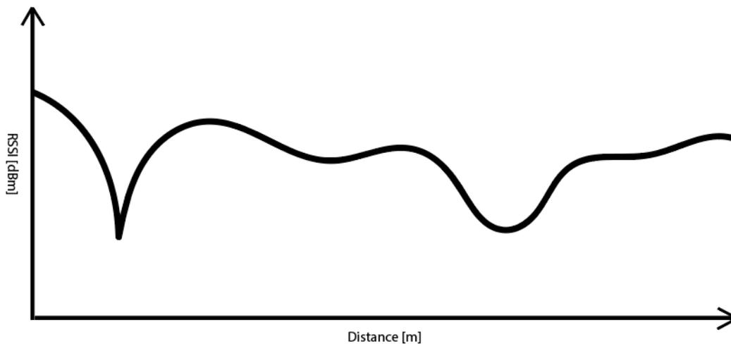
Figure 3: Signal strength in a fading environment
