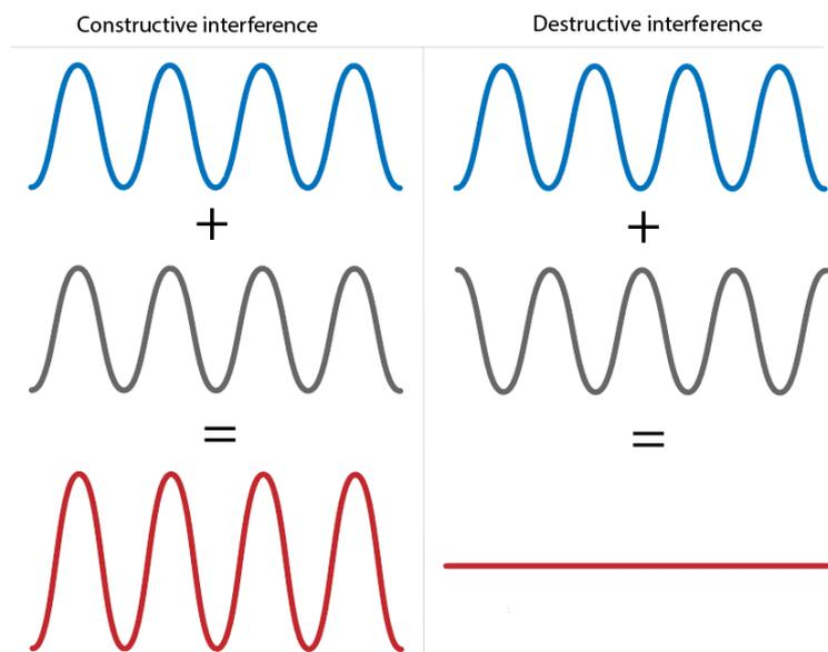
Figure 2: Constructive and Destructive interference
