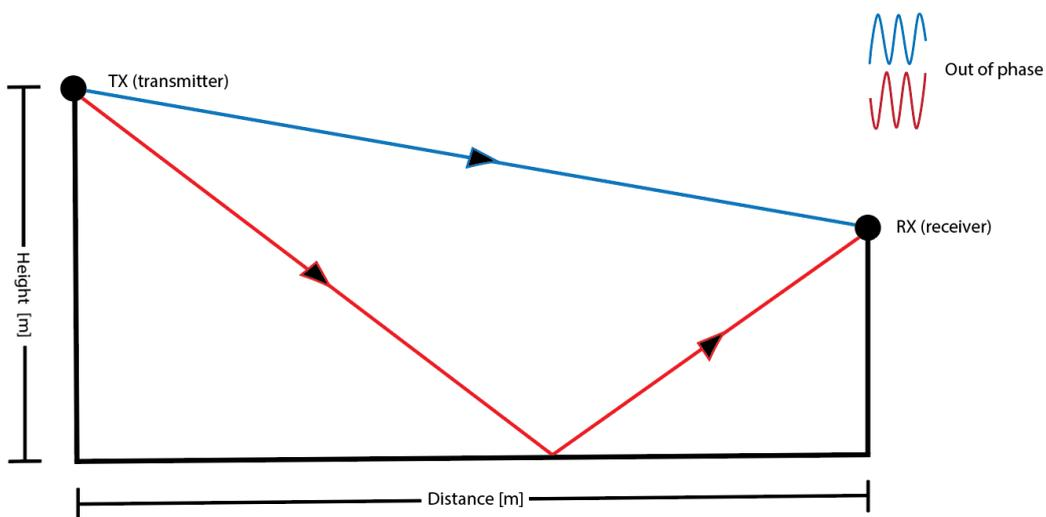
Figure 1: Ground reflection causing fading
