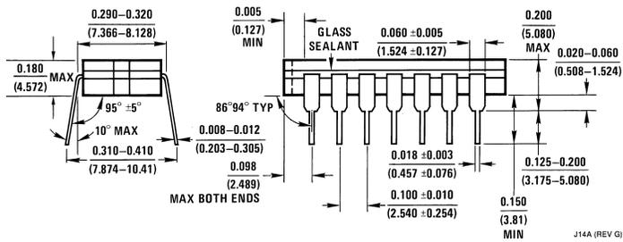
**14-Lead Ceramic Dual-In-Line Package (J)**
