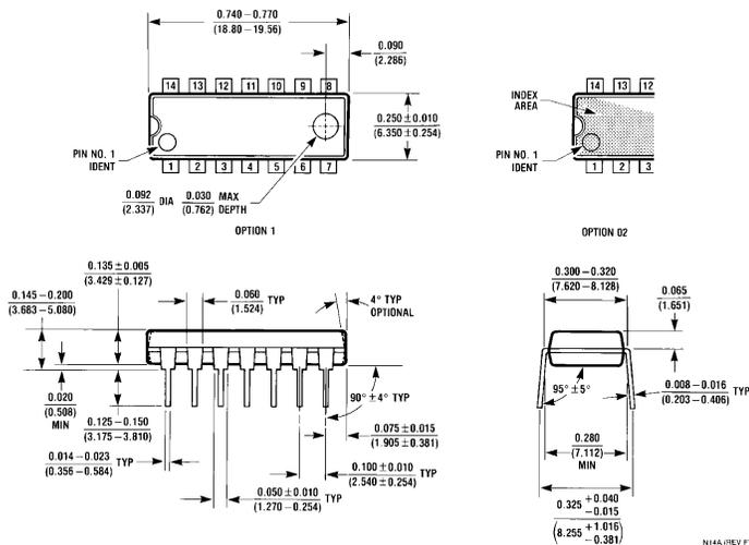
**14-Lead Molded Dual-In-Line Package (N)**
