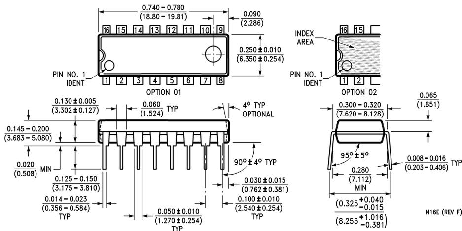
**16-Lead Molded Dual-In-Line Package (N)**
